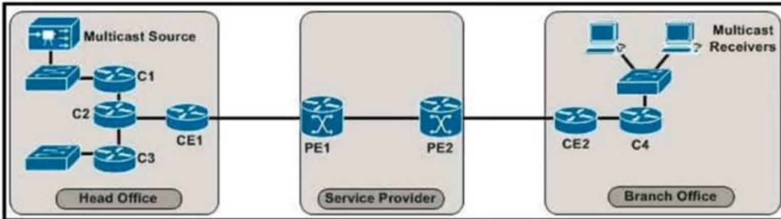
The enterprise customer wants to stream one-way video from their head office to eight branch offices using multicast. Their current service provider provides a Layer3 VPN solution and manages the CE routers, but they do not currently support multicast. Which solution quickly allows this multicast traffic to go through while allowing for future scalability?
