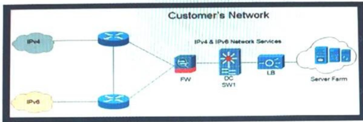
Company XYZ is currently running IPv4 but has decided to start the transition into IPv6. The initial objective is to allow communication based on IPv6 wherever possible, and there should still be support in place for devices that only support IPv4. These devices must be able to communicate to IPv6 devices as well. Which solution must be part of the design?
