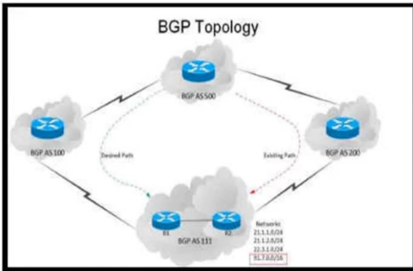
An engineer has been asked to redesign the traffic flow toward AS 111 coming from AS 500. Traffic destined to AS 111 network 91.7.0.0/16 should come in via AS 100. while traffic destined to all other networks in AS 111 should continue to use the existing path Which BGP attributes are best suited to control this inbound traffic coming from BGP AS 500 Into the 91.7.0.0/16 network?
