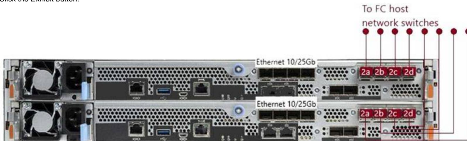
Referring to the exhibit, you installed a new AFF A250 HA system with FC at a customer site. The customer asks how many ports can be used for the Ethernet host connections.
