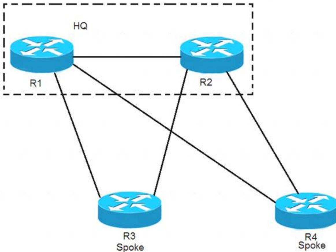
EIGRP has been configured on all links. The spoke nodes have been configured as EIGRP stubs, and the WAN links to R3 have higher bandwidth and lower delay than the links to R4. When a link failure occurs at the R1-R2 link, what happens to traffic on R1 that is destined for a subnet attached to R2?
